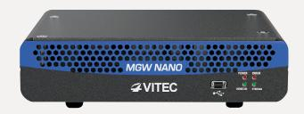
Portable MPEG-4 H.264 encoding and streaming appliance featuring Full HD processing, HD/SD-SDI and HDMI inputs, KLV / STANAG metadata support and Error-free content delivery using Zixi™ technology and ProMPEG FEC.
